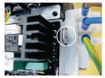
3. Install the new PCB. Insert the tenon tongue firmly into the PCB bracket. Reverse Steps 1 and 2 to fasten the PCB.
