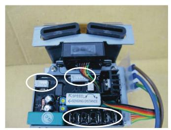
1. Disconnect all of the wires on the PCB. (See right)
