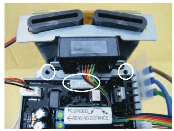
1. To change the sensor, remove the screws from the sensor bracket to take out the sensor. (See right)
