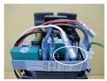
1. To change the motor, disconnect the motor wires from the PCB. (See right)
