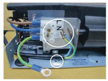
1. Disconnect the four wires and remove the ground screw. (See right)
