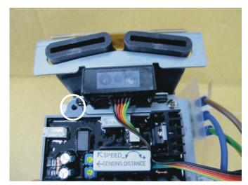
2. To change the PCB, remove the screws from the sensor bracket and the sensor. Dislodge the PCB from the PCB bracket by pushing to the left. (see right)
