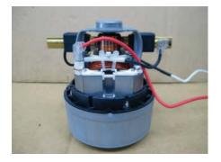
3. Remove the top housing and take out the motor. Remove and retain both motor rubbers on the top and at the bottom. Place the two motor rubbers on the new motor. Reverse Steps 1 and 2 to place the new motor firmly in the motor housing.
