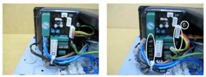
1. Pull off the six wires and remove the fixing screws of the timer.
