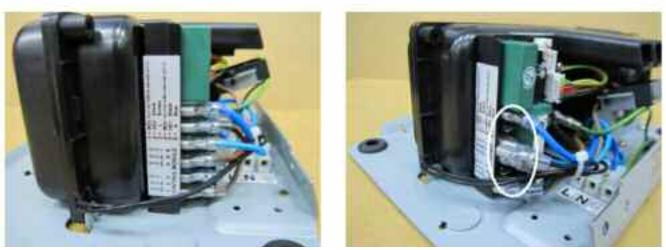
1. Remove the wires that connect heater to the timer.
