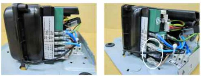
1. Remove the wires that connect motor to the timer.
