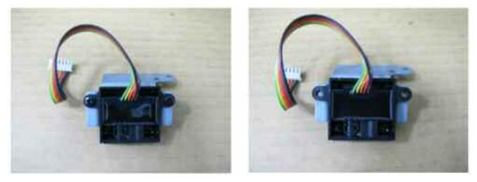
4. Remove the black screws on the sensor. Install the new sensor and reverse Steps 1~3 to fasten the sensor.
