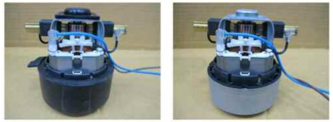
3. Remove and retain both motor rubbers on the top and at the bottom. Place the two motor rubbers on the new motor. Reverse Steps 1 and 2 to place the new motor firmly in the motor housing.
