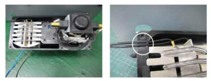
3. To replace the heater, the wire set must be fixed to the ditch in the lower housing of the blower.
