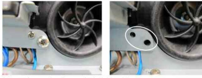
3. Remove the screws from the sensor bracket to take out the sensor.
