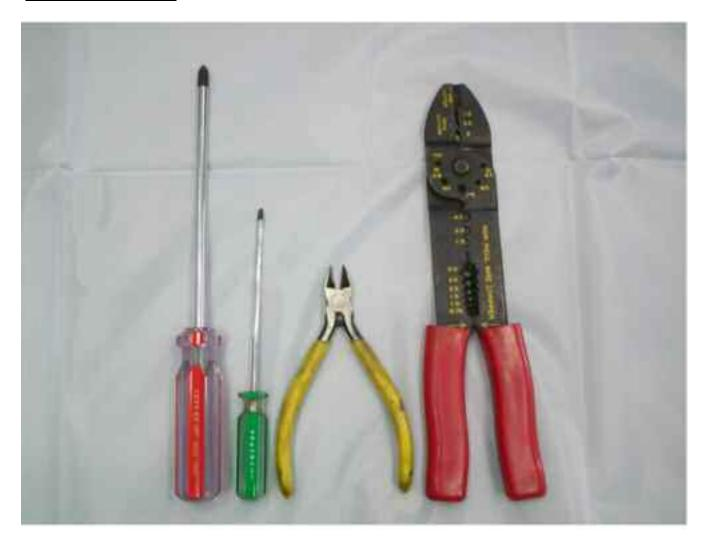
Philips Screwdriver Slotted Screwdriver Wire Cutter Modular Crimping Cuts Tool
