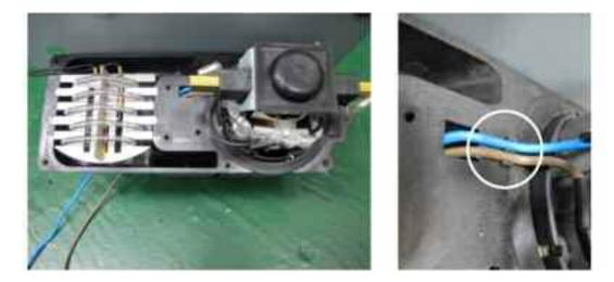
4. To replace the motor, install the motor rubber (large/small) on the motor, and place the motor under the fan blower. The wire set must be fixed to the ditch in the lower housing of the blower.
