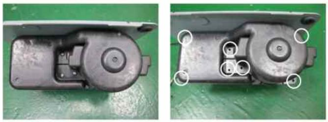
2. Loosen the fixing screws of the blower and remove the blower housing.
