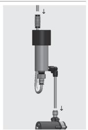
**IMPORTANT**: Make sure to cut the soap tube to the minimum required length
