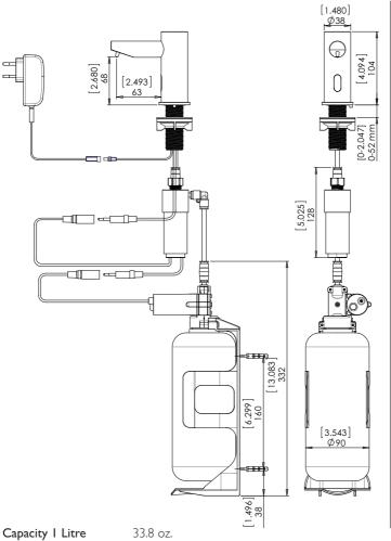
**Power Supply** 12V transformer Soap viscosity up to 100 cPs
