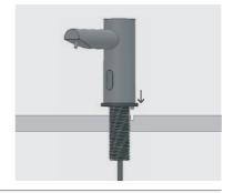
2 Under the deck, secure the gasket, disk and nut over the soap dispenser body nipple.
