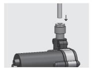
5. Connect the second soap tube provided in the packaging from the compressor to the quick connection fitting at the top of the soap dispenser pump assembly by snapping it in.
