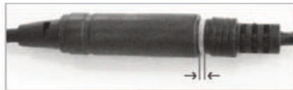
O-ring visible – not connected properly
